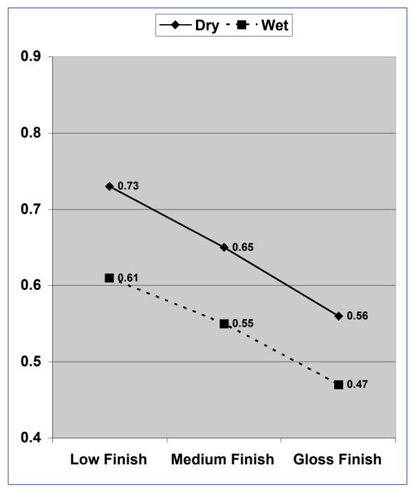
\*NOTE – According to the ADA, OSHA and ASTM guidelines, the generally accepted Safe Zone is between 0.9 and 0.5
