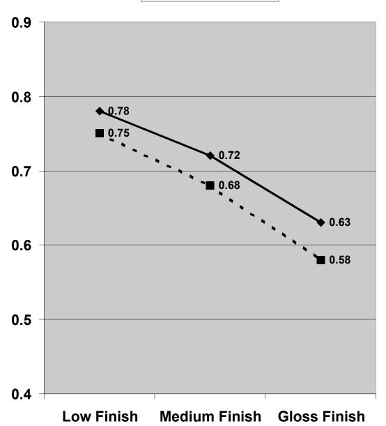
\*NOTE – According to the ADA,OSHA and ASTM guidelines, the generally accepted Safe Zone is between 0.9 and 0.5
