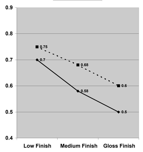
\*NOTE – According to the ADA, OSHA and ASTM guidelines, the generally accepted Safe Zone is between 0.9 and 0.5
